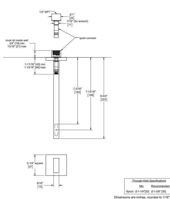
Through-Hole Specifications Min Recommended Spout: Ø1-1/4"[32] Ø1-3/8" [35]
